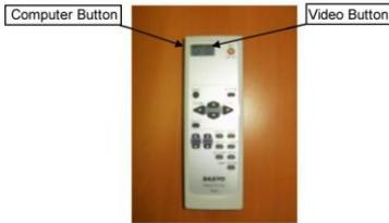
Press the video button on the projector remote to switch the input source from the DVD and Document Camera.
